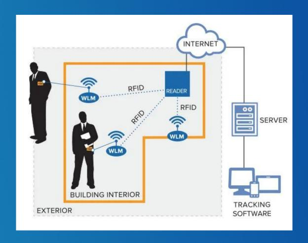
Real-time locating systems, also known as real-time tracking systems, are used to automatically identify and track the location of objects or people in real time, usually within a building or other contained area.
